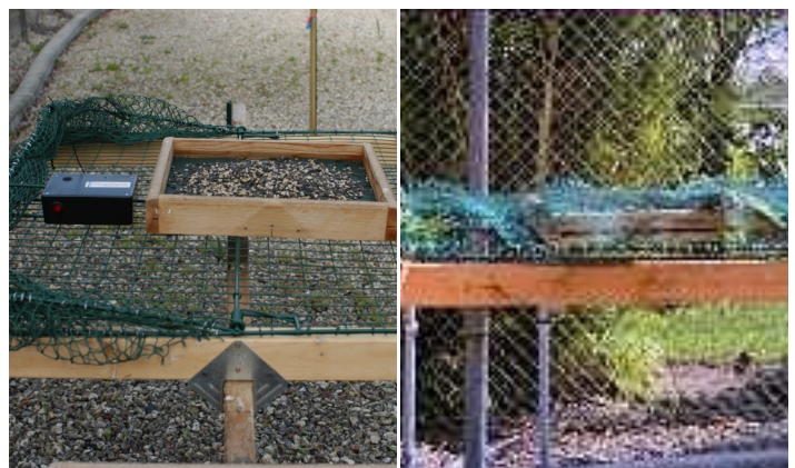
Figures 7 (left) and 8. Remotely triggered spring-loaded trap installed at monk parakeet feeding platform. After the observer confirms non-target species are not present, the trap is activated and parakeets are captured.
