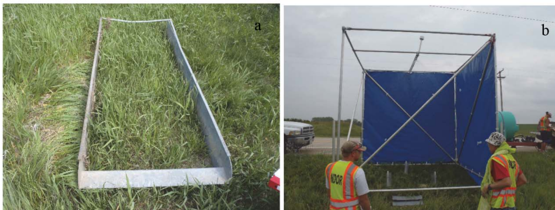
Figure 2.8 Steel frame, 3.3 ft by 1.6 ft (a) and setup (b) used for rainfall runoff collection
