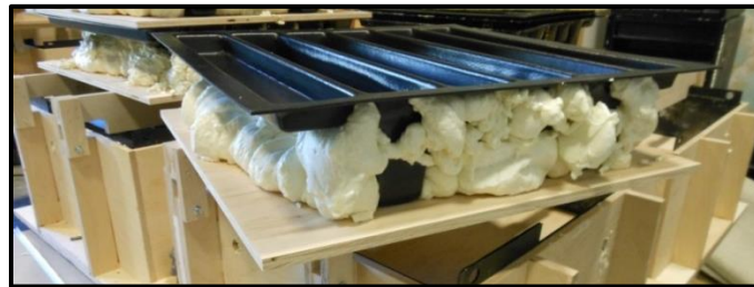
Figure 3.1.3: Acoustical Panels – Diffuser constructed with foam backing & support board
