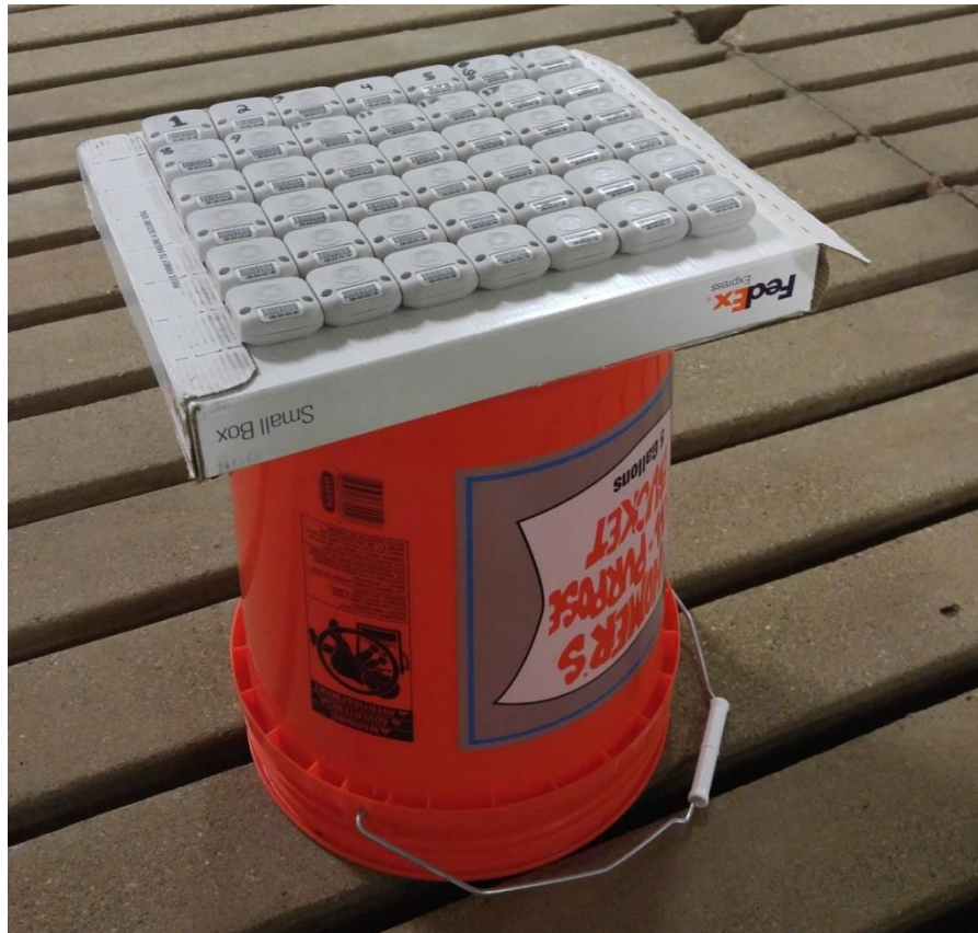
Figure 2.6 Setup for the single location test. Tags were placed on top of a bucket measuring 0.39 m in height, so that the tags would not be directly on the floor.
