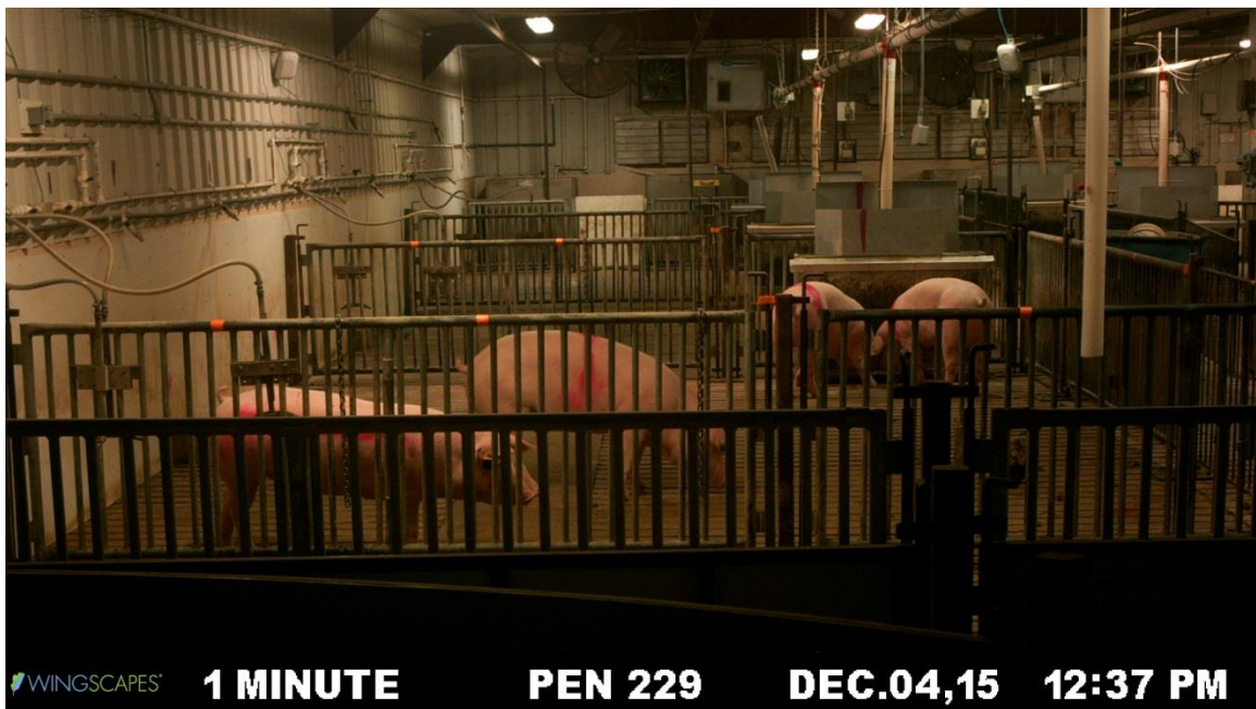
Figure 2.10 Example image along the Y axis of the swine pen. The orange tape marking 1 m intervals can be seen on the railings in the foreground and background.
