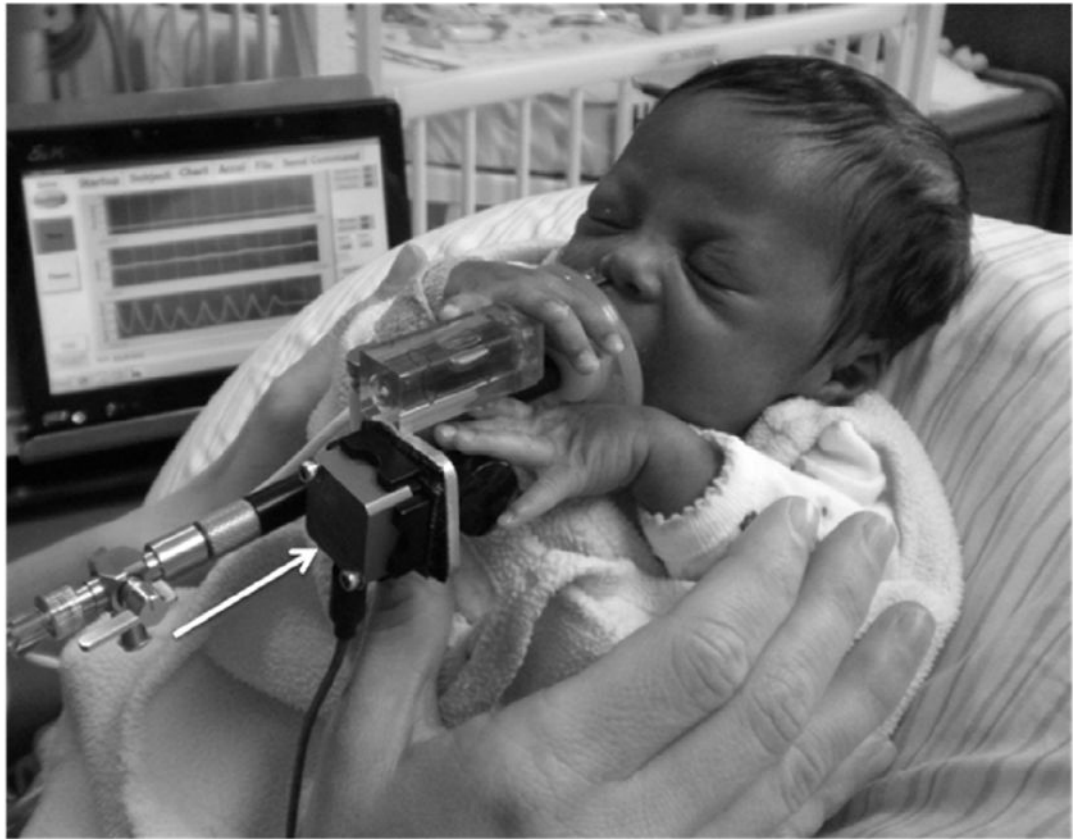
Figure 2. Infant sucking on Soothie™ pacifier during VestibuGlide stimulation. The infant's Soothie™ pacifier is attached to a Delrin receiver necessary to measure suck displacement. A uniaxial accelerometer (white arrow) was also attached to the Delrin receiver.
