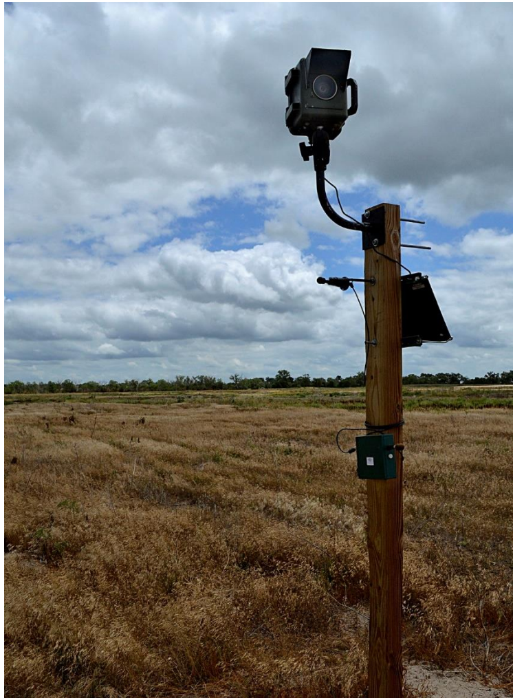
Figure 2. Digital time-lapse camera station with waterproof housing and solar panel.
