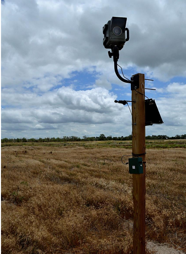
Figure 2. Time-lapse camera system with solar panel owned by Platte Basin Timelapse in the central Platte River Basin
