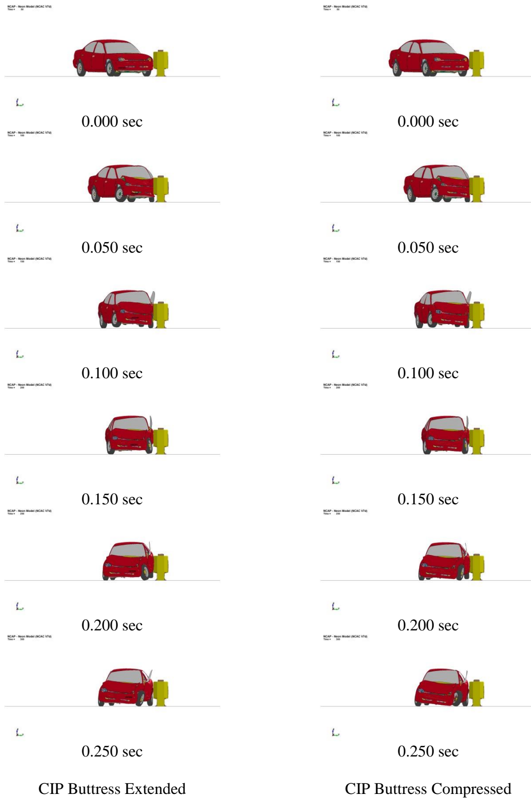
Figure 150. RESTORE Barrier Transition, 1100C Neon Simulation Comparison, CIP Locations, Downstream View
