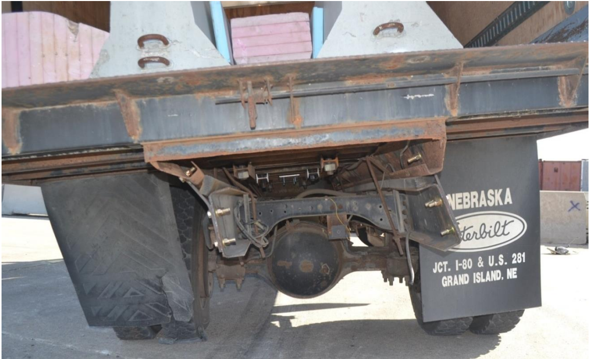
a. Full-Scale Test Box Attachment Damage
