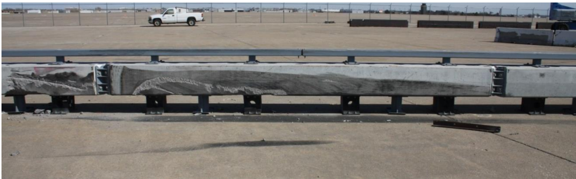
Figure 42. RESTORE Barrier Damage, Test No. SFH-3 [20-21]
