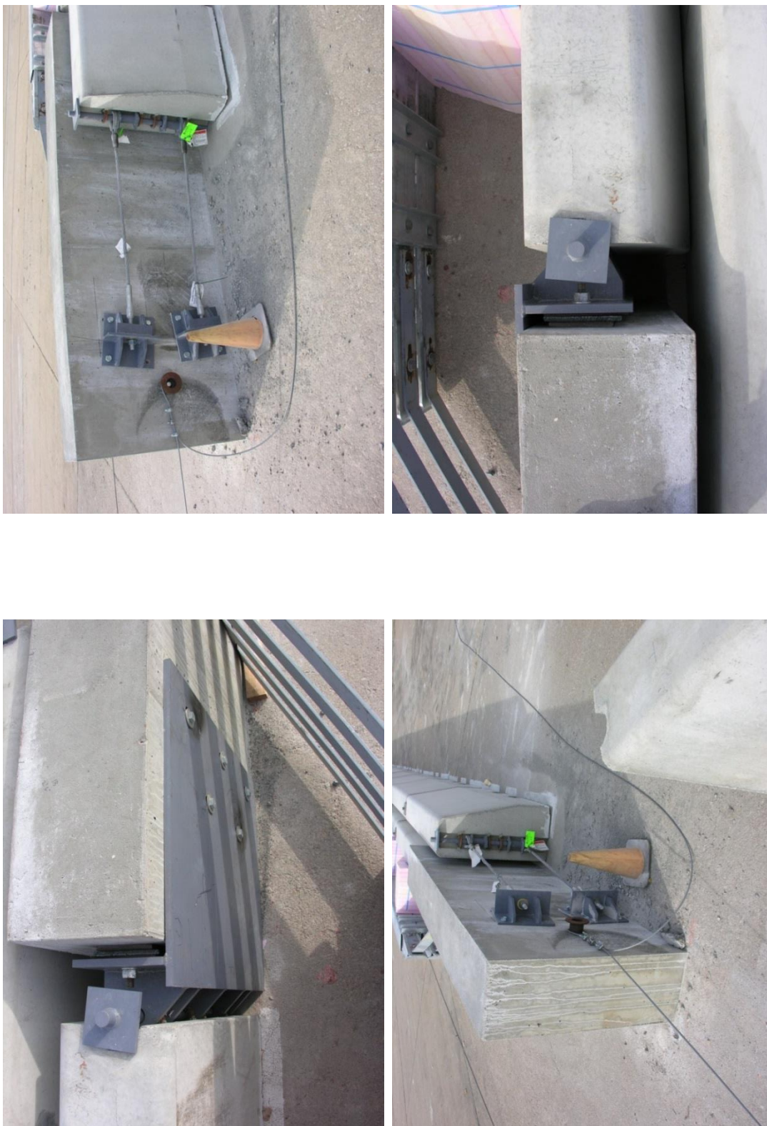
Figure 17. Pre-Test Photographs of SAFER on PCB Installed Across Opening, Test No. SPCB-1 [39-40]
