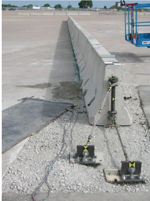
Figure 10. Portable Concrete Barrier (PCB) Anchorage and Termination [31-32]
