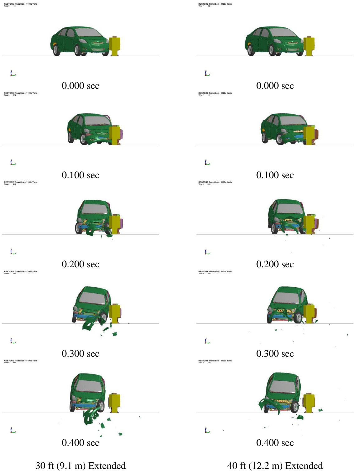
Figure 162. RESTORE Barrier Transition, 1100C Yaris Simulation Comparison, Upstream Impact Locations, Downstream View
