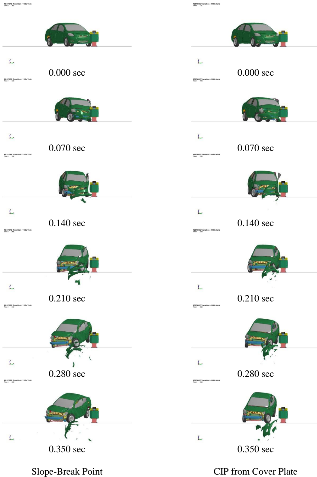
Figure 182. RESTORE Barrier Transition, 1100C Yaris Simulation Comparison, Reverse-Direction Locations, Downstream View
