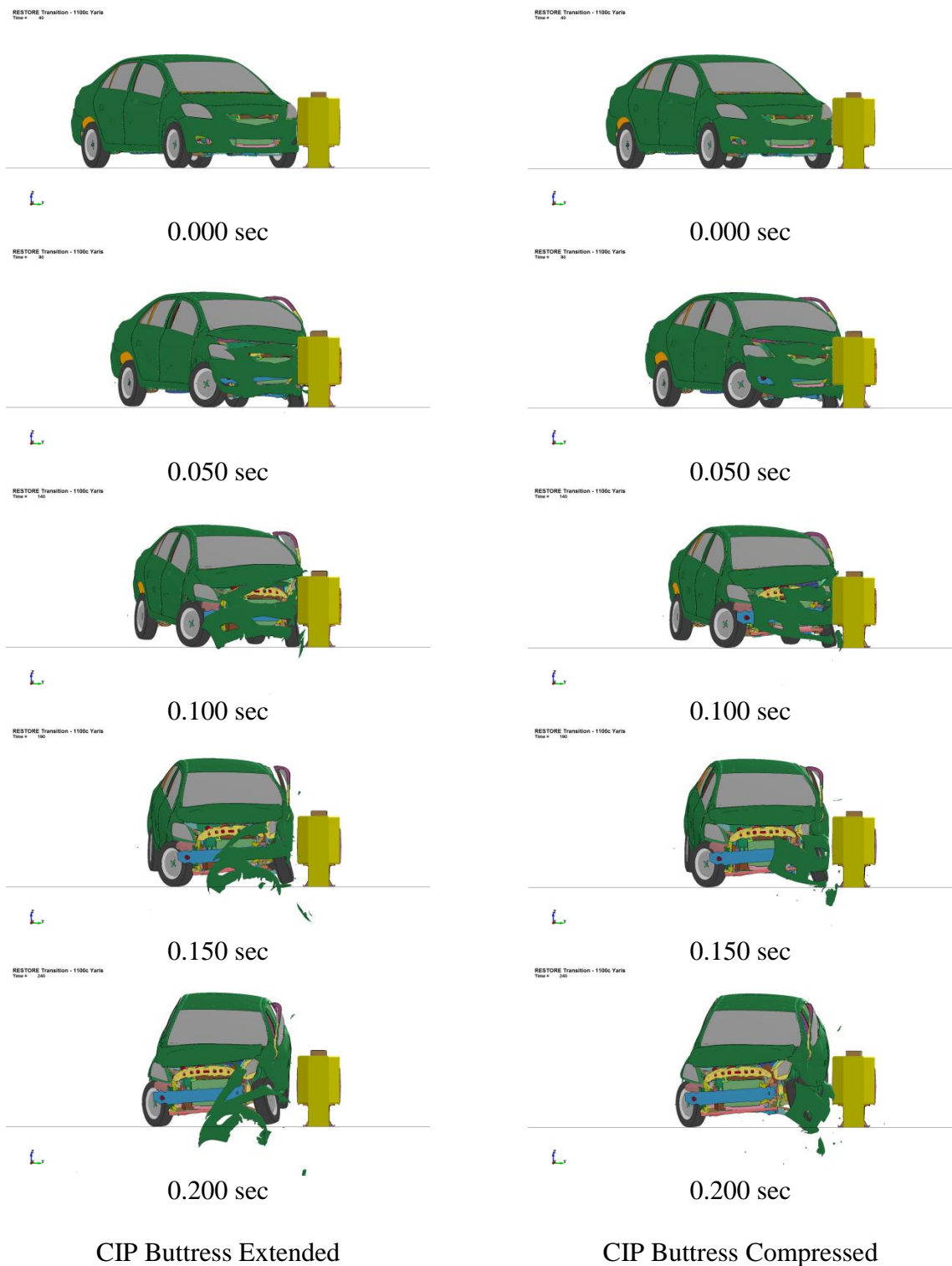
Figure 138. RESTORE Barrier Transition, 1100C Yaris Simulation Comparison, CIP Locations, Downstream View
