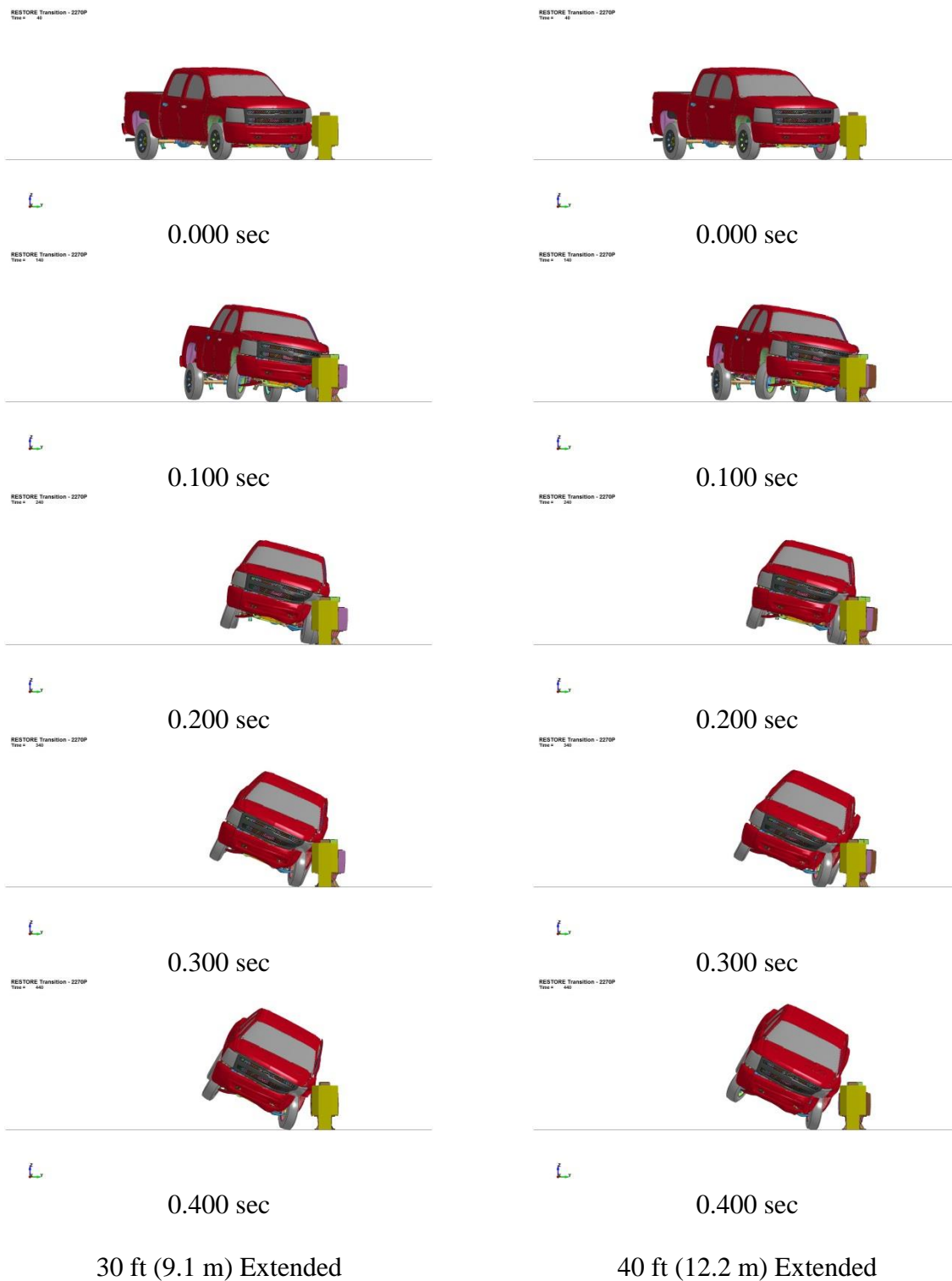
Figure 212. RESTORE Barrier Transition, 2270P Silverado Simulation Comparison, Upstream Impact Locations, Downstream View
