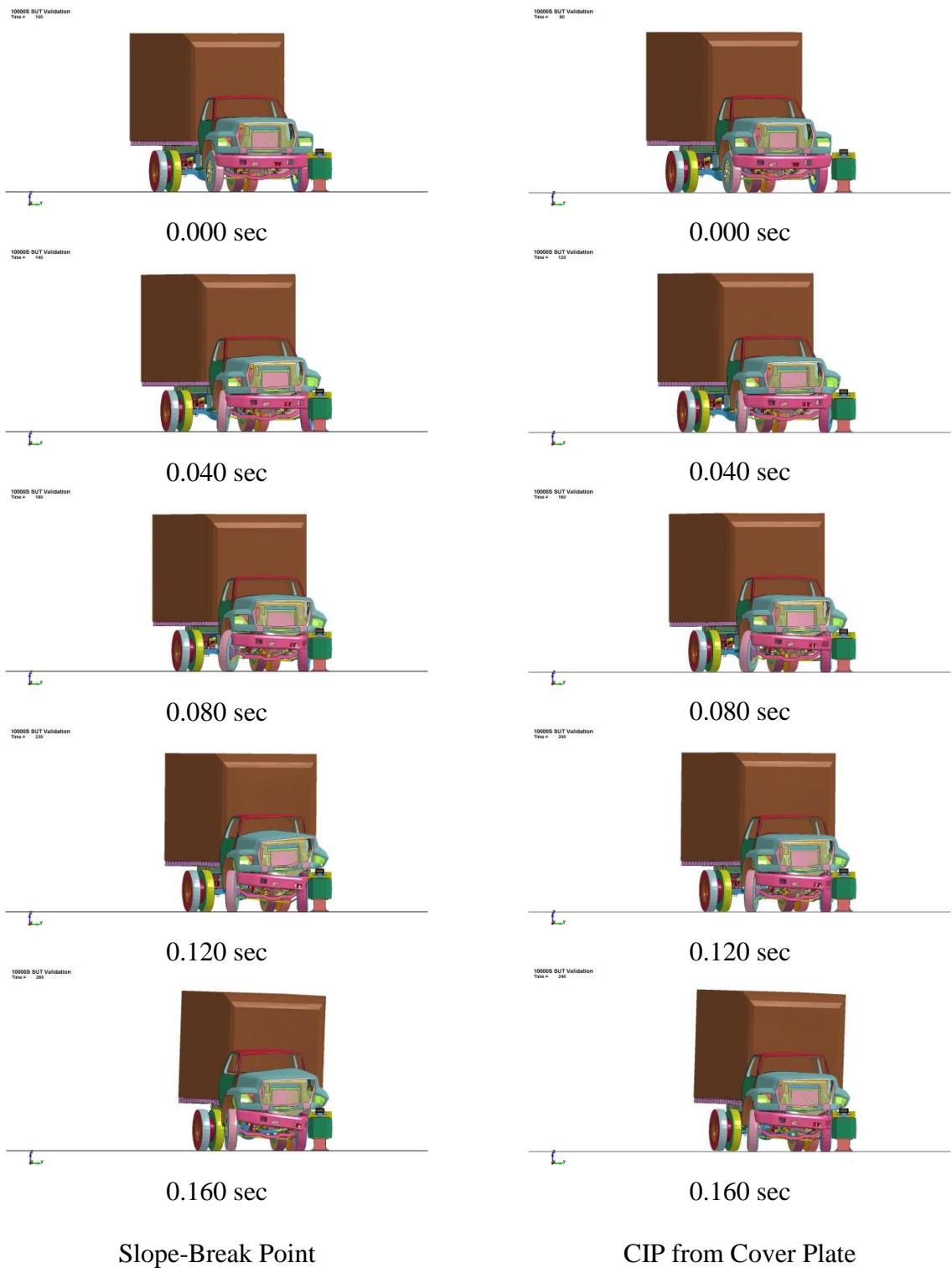
Figure 254. RESTORE Barrier Transition, 10000S F800 Simulation Comparison, Reverse-Direction Locations, Downstream View
