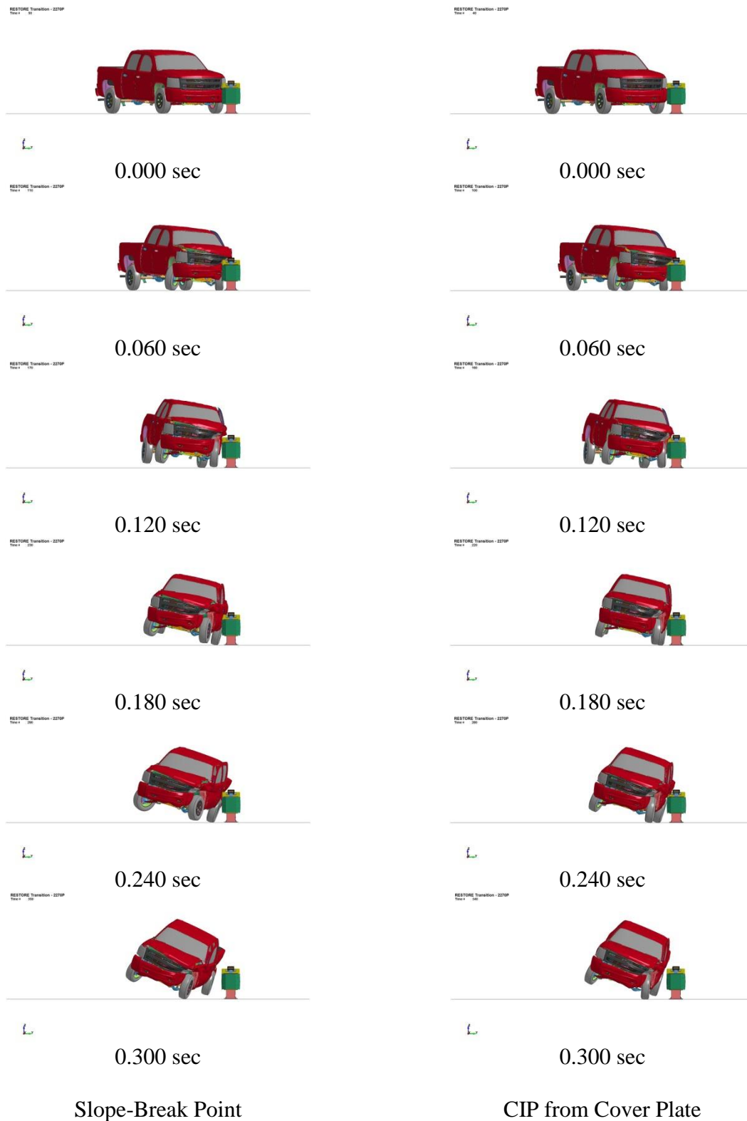
Figure 221. RESTORE Barrier Transition, 2270P Silverado Simulation Comparison, Reverse-Direction Locations, Downstream View
