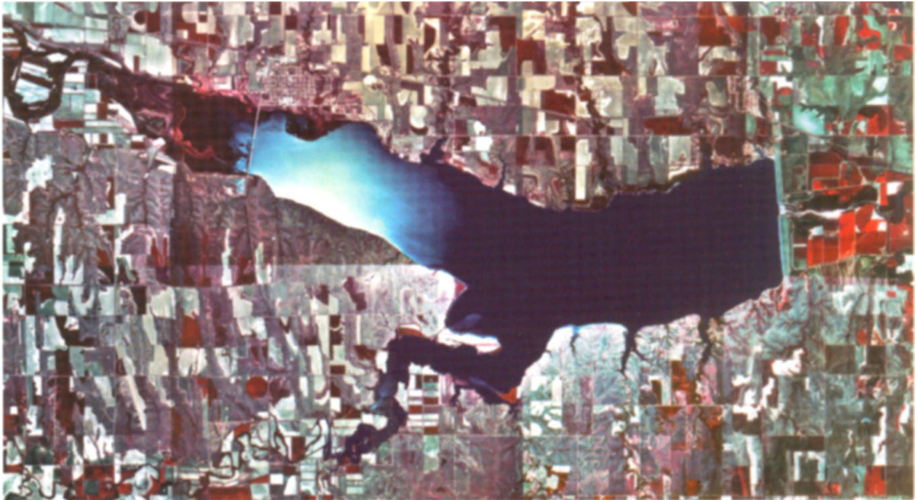
Fig. 5. Color infrared aerial photograph of Harlan County Lake area in 1988 after dam construction. Healthy vegetation appears red; dormant areas are gray-green. Water appears blue to black (CALMIT image).
