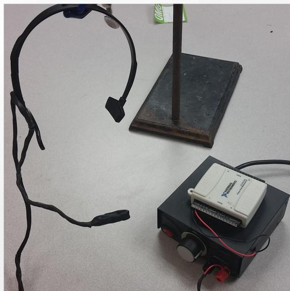
Figure 1. Hotwire anemometer and power source
