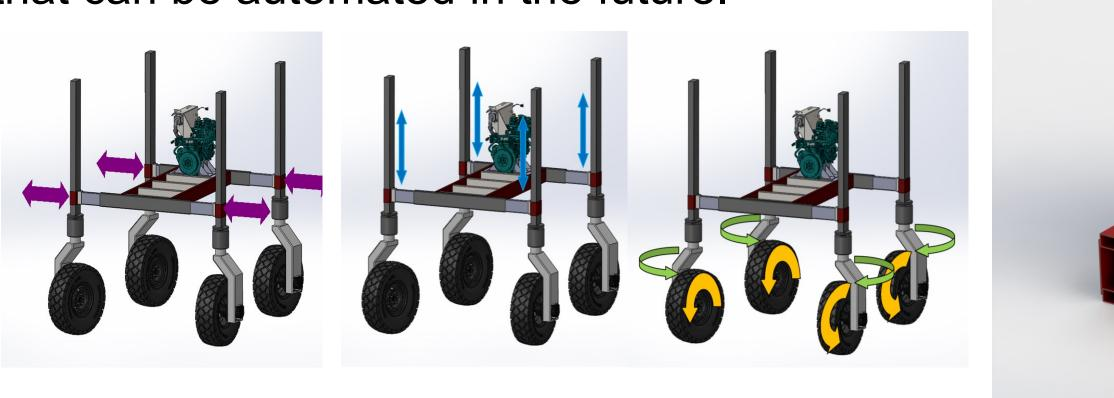
**<u>Drivetrain</u>**: A Kubota 57HP gasoline engine (WG1605-GL-E3-KEA-1, Kubota), which powers an H1 Series Danfoss tandem hydrostatic pump powers the machine. The flexible structure requires each wheel to be independently driven and steered. Four fixed displacement hydraulic motors, one for each wheel, are engaged by the pump.
