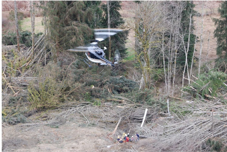
Figure 5. Extraction flight showing the low altitude of the helicopter and risk to personnel on the ground from a crash. Courtesy of Northwest Regional Aviation.
