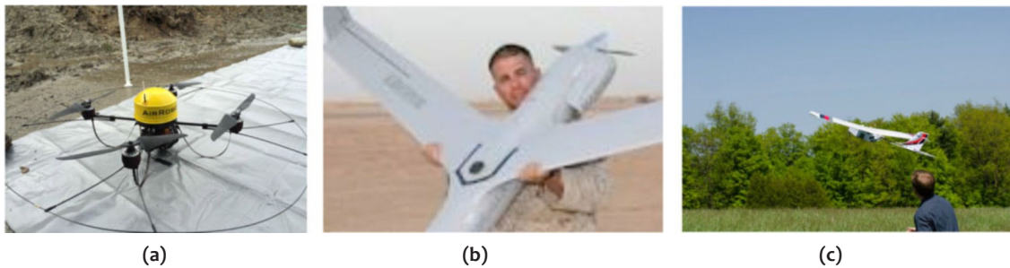
Figure 2. Roboticists Without Borders platforms selected for deployment: (a) the AirRobot AR100B, (b) the Insitu Scan Eagle, and (c) the PrecisionHawk Lancaster.
