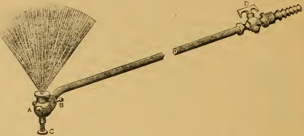
FIG. 224.—Attachment for underspraying certain garden plants.
