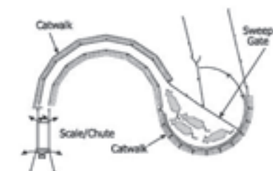
FIGURE 3. Handler movement pattern for use in a curved chute system. The techniques here and in Figure 2 make it possible to greatly reduce or eliminate electric prods. http://www.grandin.com/references
