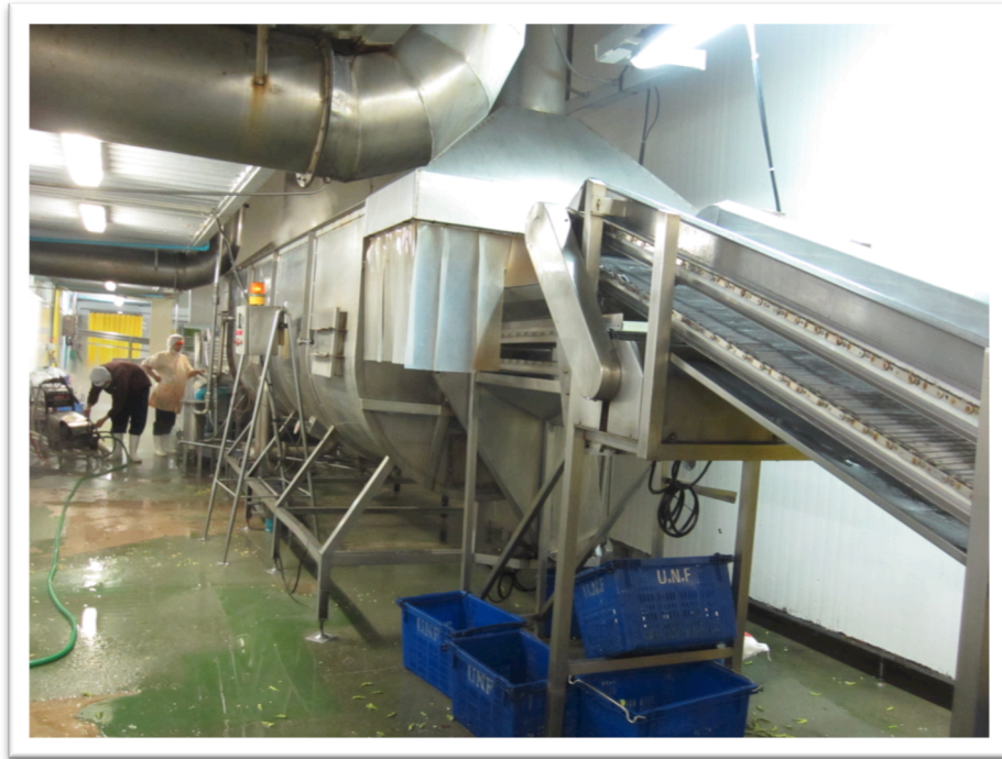
Figure 1. Rotary drum blancher (Suwit Machinery, Lamphun, Thailand)
