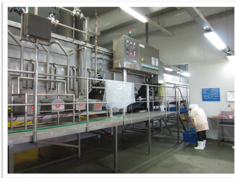
Figure 2. Continuous steam blancher (JV industrial Co. Ltd., Bangkok, Thailand)
