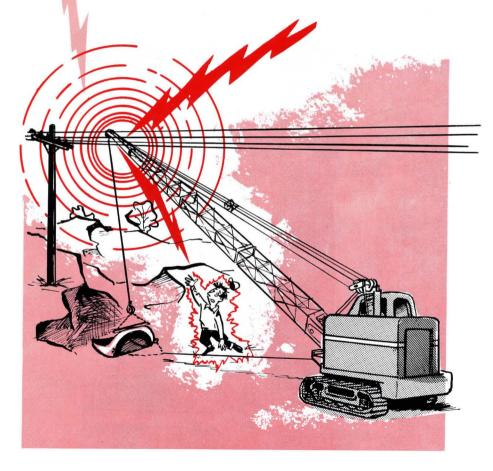
Well drilling rigs operated close to power lines cause many deaths in Nebraska. Never let the equipment come near these wires. Remember, it's the worker on the ground who usually is hurt. Be sure that the machine is out of reach of power lines when you are repairing and cleaning it.
