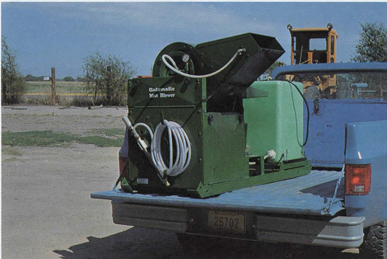
Fig. 14.—Mist blower for knockdown spray
