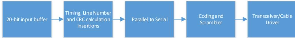
Figure 18: HD-SDI Transmitter Block Diagram
