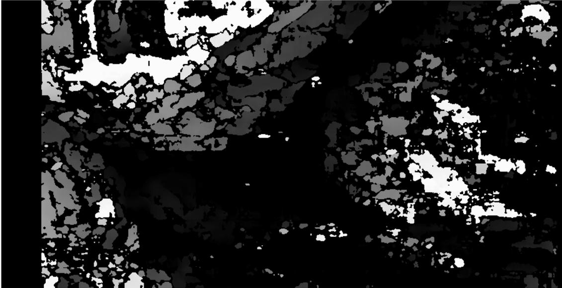
Figure 43: Resulting disparity map generated from rectified images using stereo matching.
