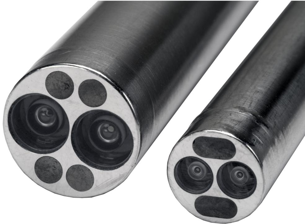
Figure 15: 12mm and 8.5mm endoscopic tip from da Vinci Si surgical robot.
