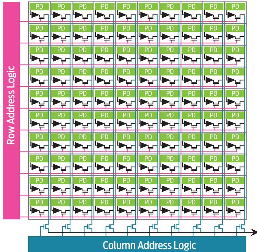
Figure 5: CMOS sensor diagram
