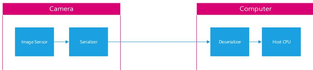
Figure 17: Block diagram illustrating the process of transmitting camera data to a computer over a serial link.
