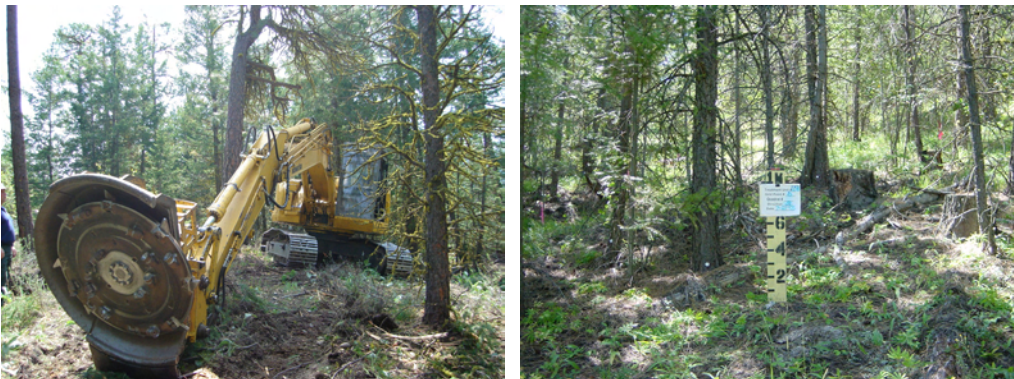
Figure 1. Mastication equipment used in the current study (left photo) and a pre-treatment stand to be thinned (right photo).
