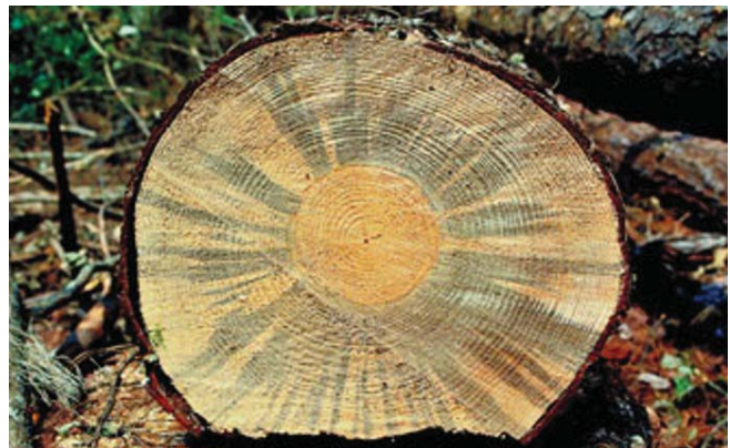
Pine killed by beetle with blue stain fungus, cross section of a log. Credit: Ronald F. Billings, Texas Forest Service, www.Bugwood.org .
