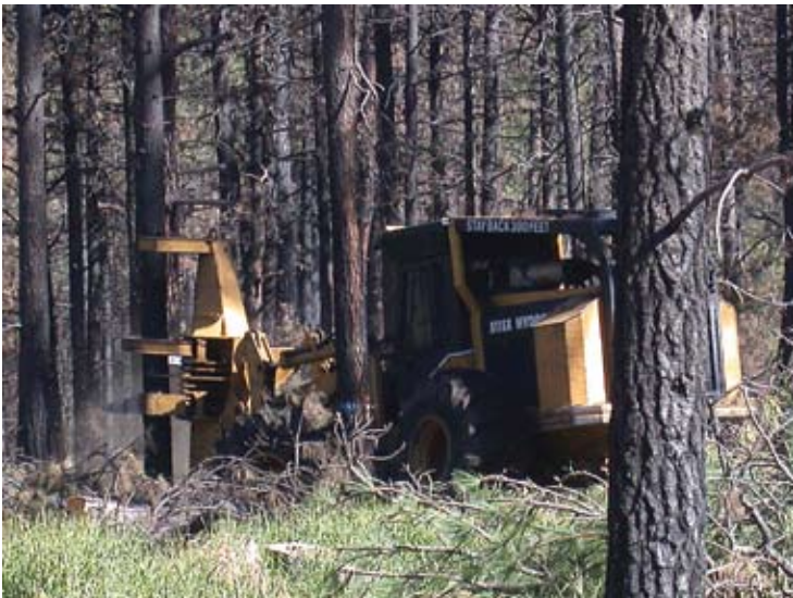
Figure 23. Feller-buncher head attached to a rubber-tired prime mover. Photo credit: Molly Hunter.
