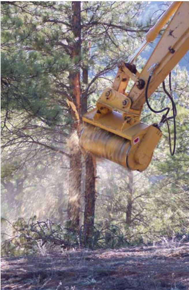
Figure 28. Example of a vertical shaft masticator, a Quadco© brush cutter on a Timbco© tracked harvester. Photo credit: Kristen Garrison.
