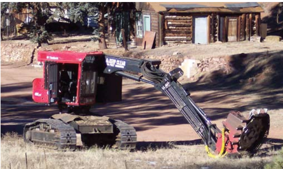
Figure 29. Example of a horizontal shaft masticator, a Wag Way© drum grinder. Photo credit: Kristen Garrison
