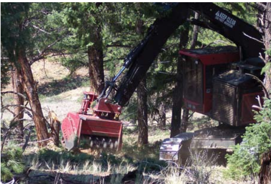
Figure 24. Mastication head attached to a boom or articulated arm of a Timbco© tracked timber harvester. Photo credit: Kristen Garrison.
