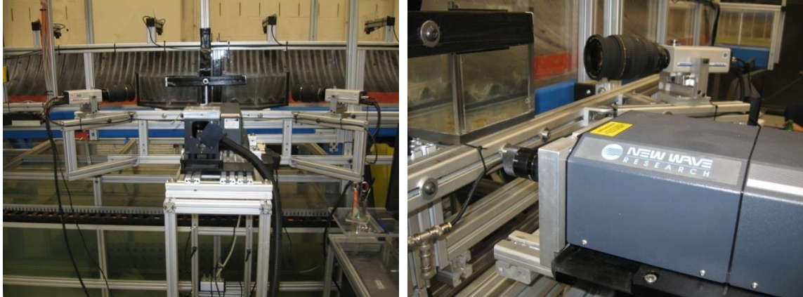
Figure 3.2 S-PIV Setup a) Front View b) Side View
