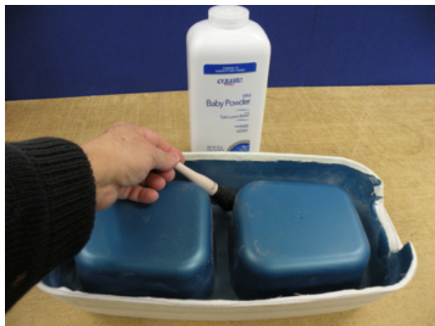
Use a small brush or cotton ball to apply a very thin dusting of talcum powder to the trap.
