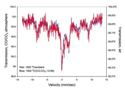
Fig. 4. <sup>57</sup>Fe Mössbauer spectra of glasses melted at 1500 °C in air (red) and under 12CO/88CO<sub>2</sub> reducing atmosphere (blue).
