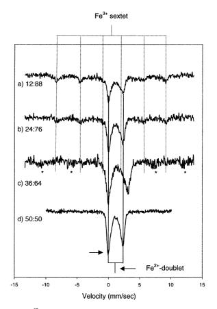
Fig. 5.  ${}^{57}$ Fe Mössbauer spectra of glasses melted at 1500 °C in air under reducing atmospheres of (a) 12CO/88CO<sub>2</sub>, (b) 24CO/76CO<sub>2</sub>, (c) 36CO/64CO<sub>2</sub>, and (d) 50CO/50CO<sub>2</sub>.
