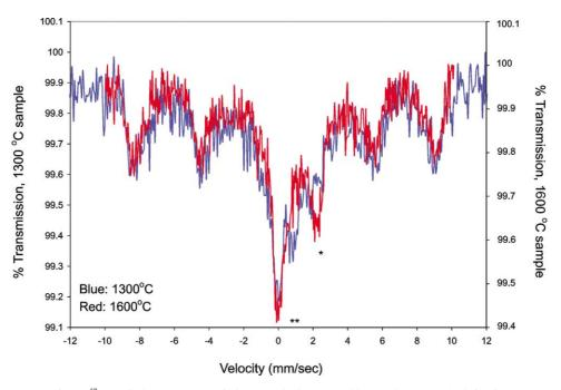
Fig. 3. <sup>57</sup>Fe Mössbauer spectra of glasses melted at 1300 (blue) and 1600 °C (red) in air.
