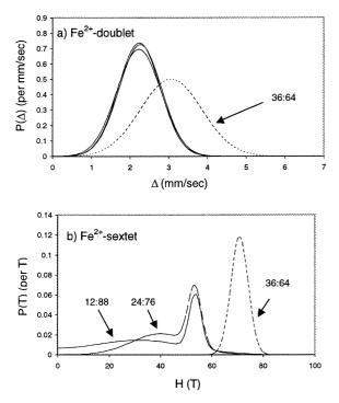
Fig. 9. QSD and HFD distributions of Fe-sites for the glasses melted for the glasses melted in  $CO/CO_2$  atmosphere (12/88 to 50/50).
