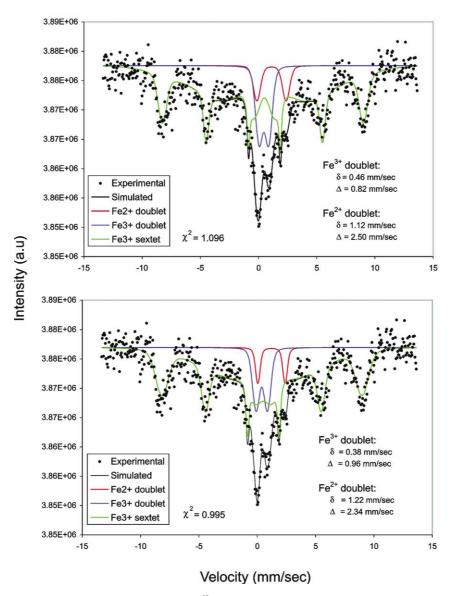
Fig. 7. Model simulation comparison based on 4.2 K <sup>57</sup>Fe Mössbauer spectrum of the glasses melted at 1300 °C in air.
