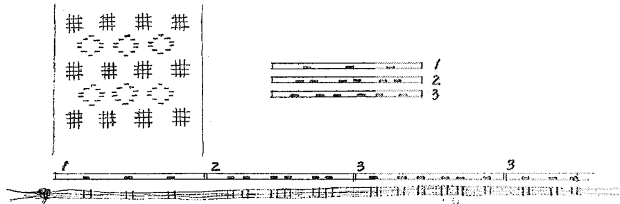
Fig.9. The koba jogi , used for creating pictorial weft kasuri. The design is painted on stacked boards.
