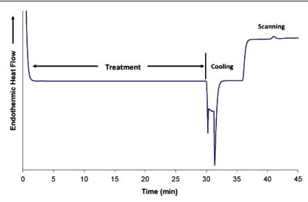
Figure 1. Sample treatment and scanning by DSC. Samples were treated at specific temperatures for 30 min, followed by cooling and scanning.
