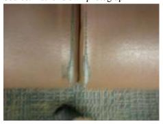
Figure 12-Fabric finish wearing off at seam.
