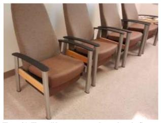
Figure 21- These gliders are open underneath so the floor can be cleaned without moving them. The metal legs are not as easily damaged by vacuums or buffers.
