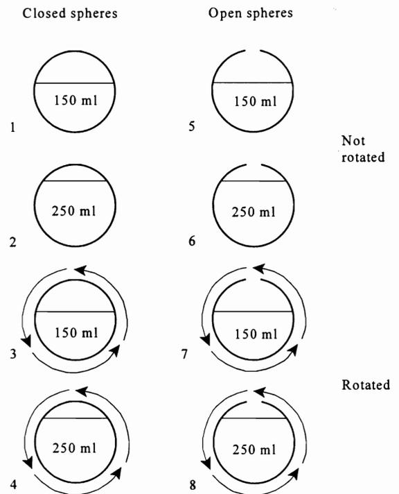
Figure 1. Biosphere treatments for the  $2 \times 2 \times 2$  factorial design replicated once ( $N = 16$ ). This design produced eight unique treatments by the biosphere combinations shown above.
