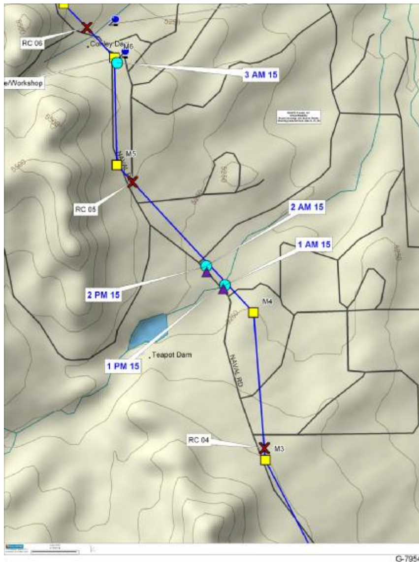
Figure 8. Positions of two adjacent leaks present both Wednesday AM and PM show resolving power.
