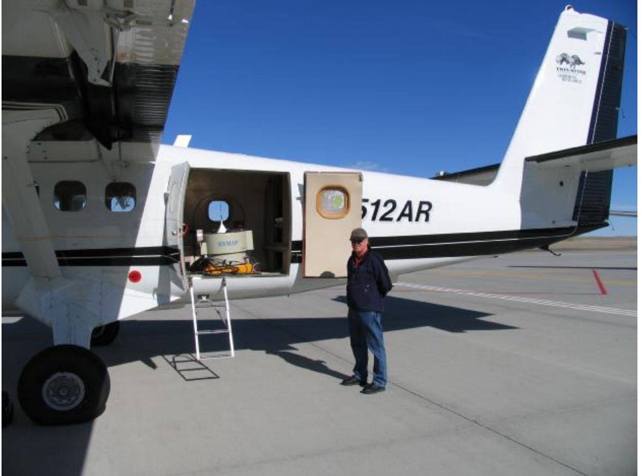
Figure 1 The HyMap sensor is white sitting on the stabilizing platform that is yellow inside the Twin Otter manned aircraft. Mike Hornibrook who is the HyVista operator is shown standing outside side the hatch doors.
