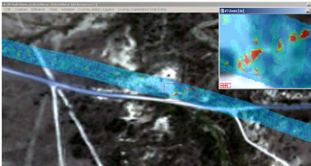
Figure 1.1.3 Visual Display of Natural Gas Emissions Detected By the ANGEL System on the Afternoon of September 17 th , 2004 (Calibration Leak)
