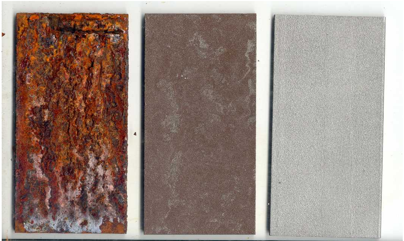
1 WEEK EXPOSURE TO PROHESION CYCLE
