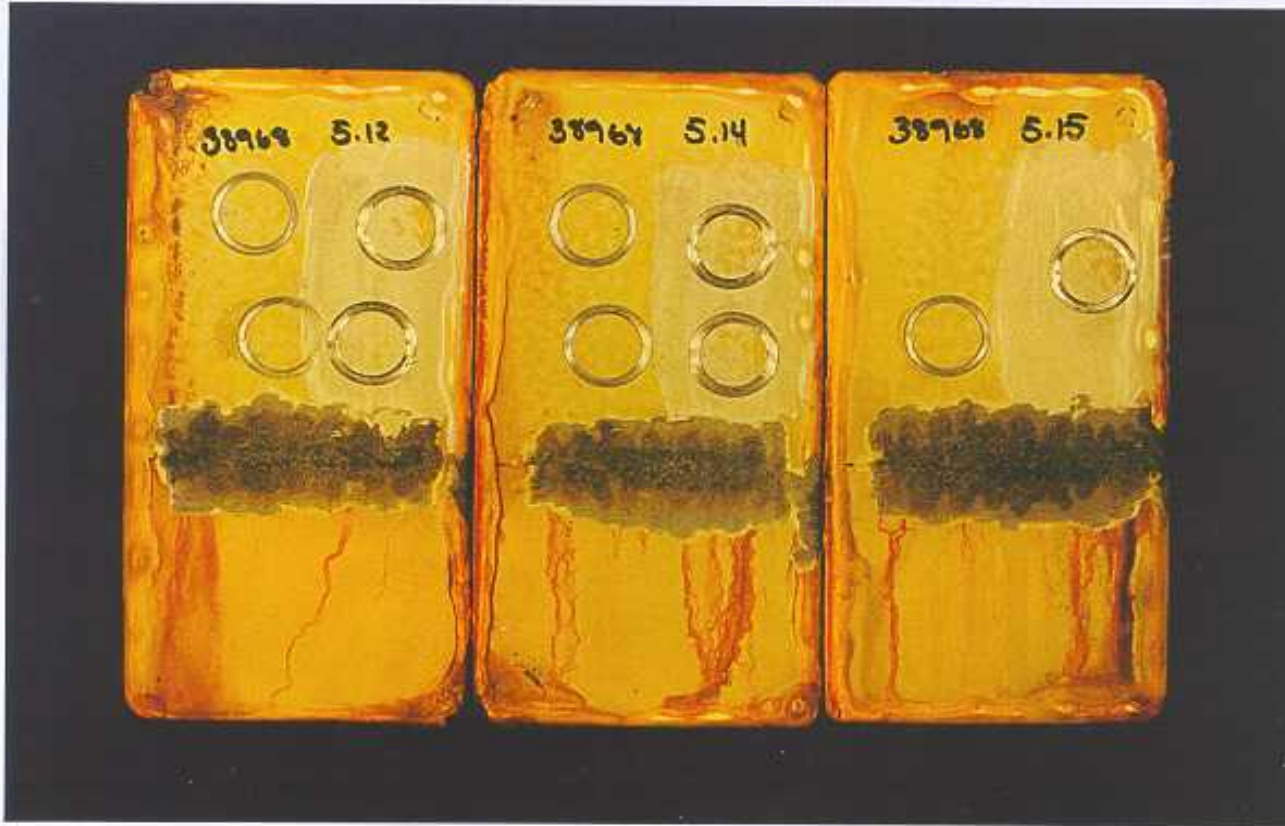
Photo no. 1. Panels after Cyclic salt spray / UVA test
