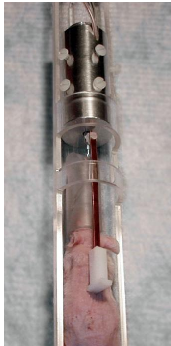
Figure 23. Potential in vivo piezoelectric stack actuator system. The MRE probe will be capable of high resolution elasticity analysis at frequencies greater than 2.5 kHz.
