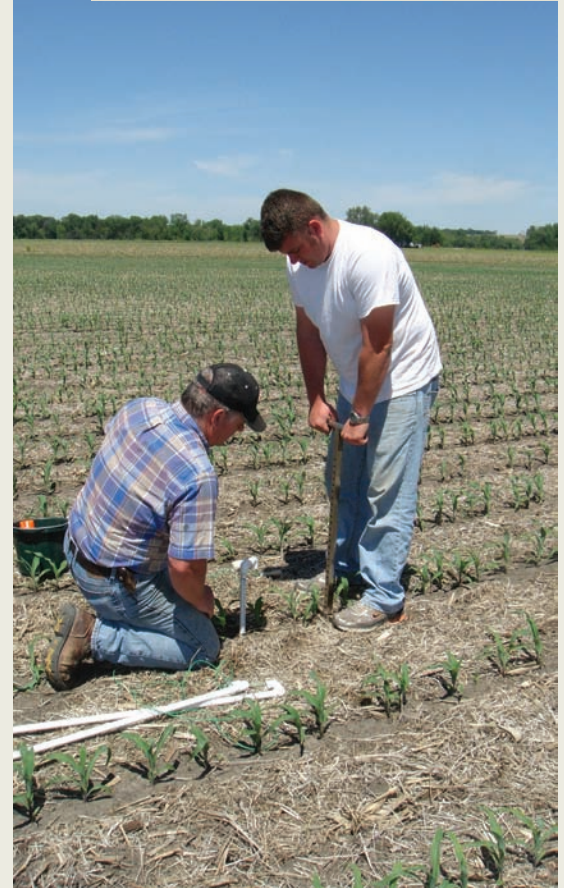
Jack Mulliken and his son Robert install Watermark soil moisture sensors near Nickerson.
