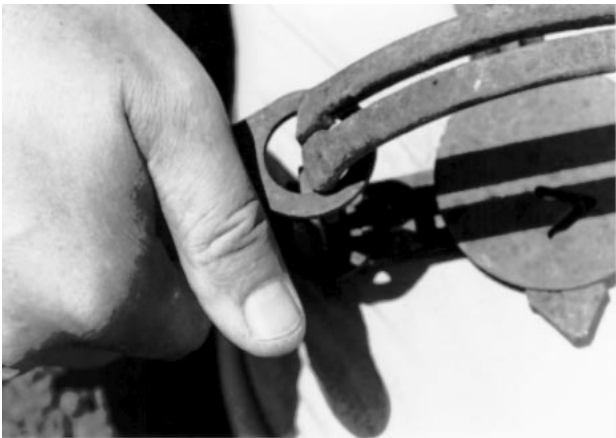
Fig. 13. Place one of the traps on your left leg just above your knee. Grasp the trap spring nearest your right leg as shown, and compress the spring.
