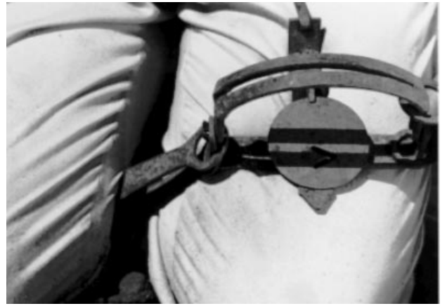
Fig 15. Hold the compressed spring with your right leg as shown above, then compress the left spring. Hold this spring down with your left hand.
