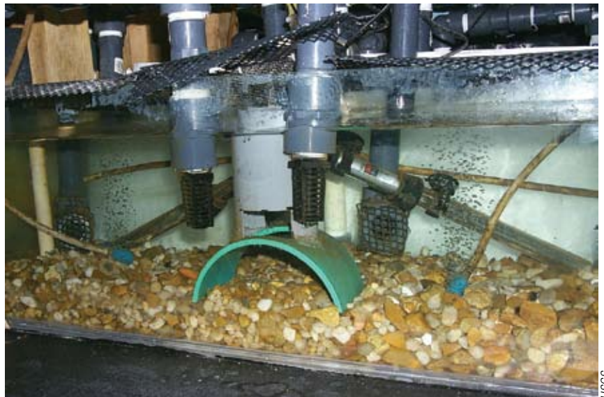
This experimental tank equipped for controlling temperature, flow, and photo-period in Neosho madtom research is monitored by external and underwater cameras.
