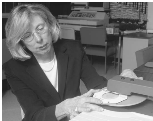
Textile Scientist Patricia Crews measures the Ultraviolet Protection Factor of a knitted fabric being considered for sun-protective clothing.
