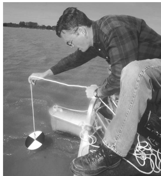
Tadd Barrow, a water resources specialist, uses a Secchi disk to measure water clarity on a lake near Beatrice.
