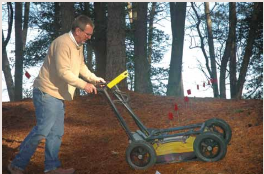
Ground-penetrating radar is being used to scan cemetery grounds at Chincoteague National Wildlife Refuge, VA and identify burial sites. (USFWS)
