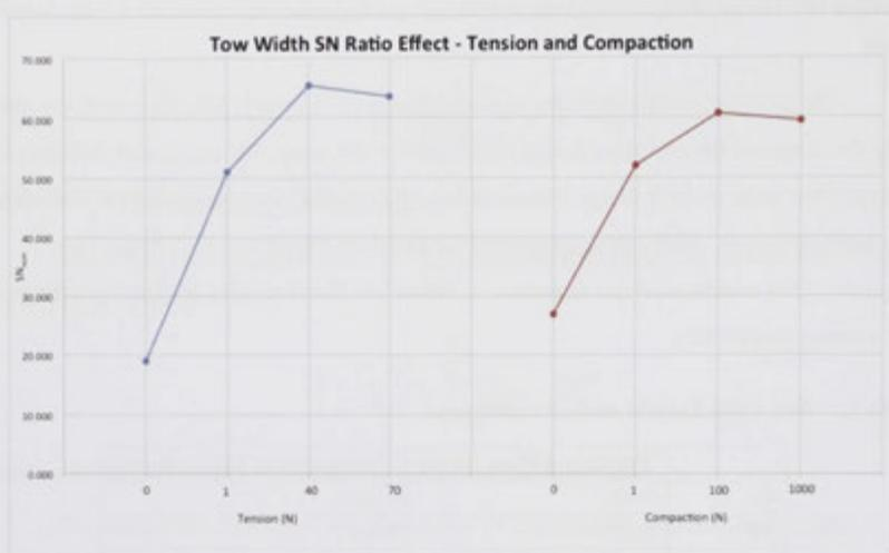
Figure 56 – Tow width signal to noise effect response
