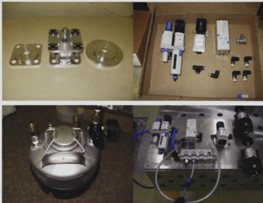
Figure 144 – The pneumatic compaction actuation platform (top left), pneumatic compaction control system (top right), the resin spray tank (bottom left), the mounted pneumatic control system
