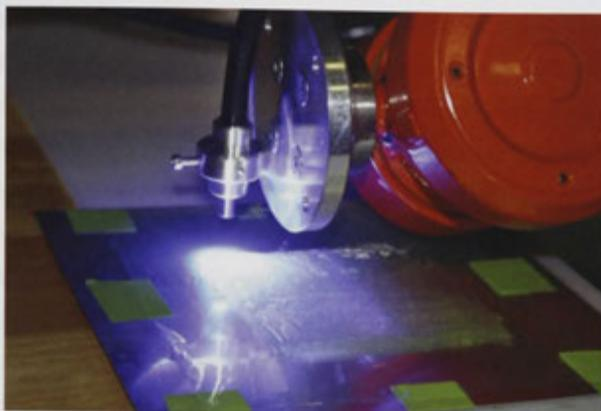
**Figure 116 – Image of the UV light mounted onto the end of an ABB IRB1600 industrial robot passing over the laminate**
