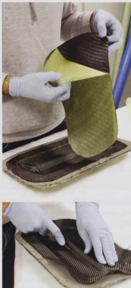
**Figure 4 – Manual prepreg lay-up**
