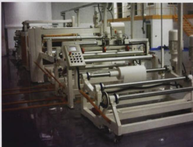
**Figure 83 – A preimpregnating machine used for coating woven and unidirectional textiles such as composite fibre reinforcements**
