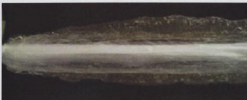
**Figure 103 – Excess resin bleed in impregnation trials**
