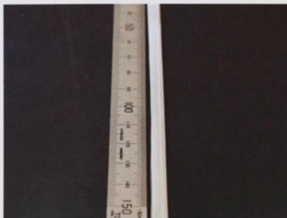
**Figure 62 – Dry glass fibre tow “straightness” test for single tow placement**
