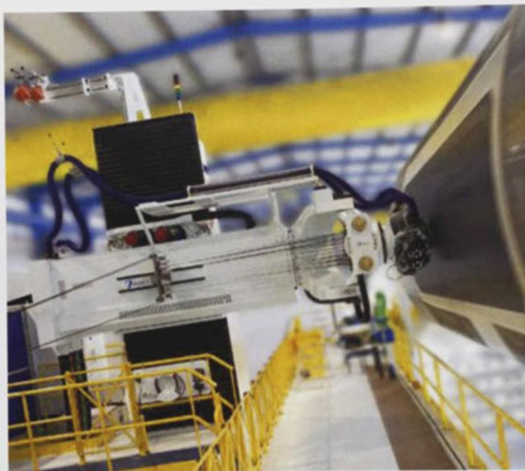
**Figure 13 - Automated fibre placement machine TORRESFIBRELAY-UP.**
