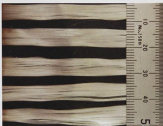
**Figure 61 – Photographic width measurements of OCV Advantex Single End Roving Type 30 glass fibre tows**
