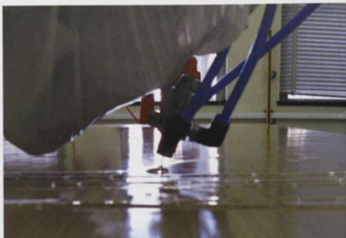
**Figure 101 – Resin flow rate calibration trials using the robotised setup**
