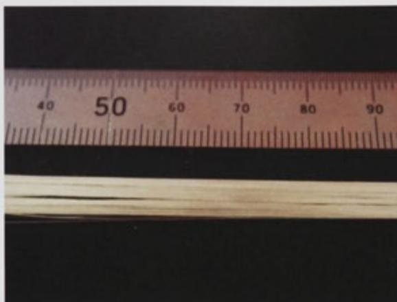
**Figure 63 – Tensioned and compacted fibre tow with a very small amount of resin cured to fixed the stack in the ‘as applied’ form. Note the gap in the tow and stringer filaments**
