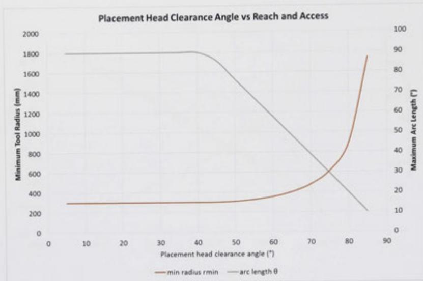
Figure 27 – Placement head clearance angle versus minimum tool radius and maximum arc length
