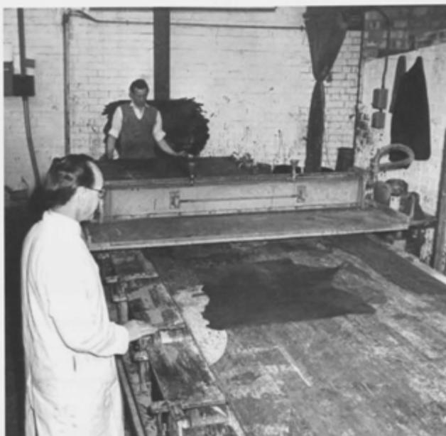
Figure 84 – Manual curtain coating being used in leather impregnation
