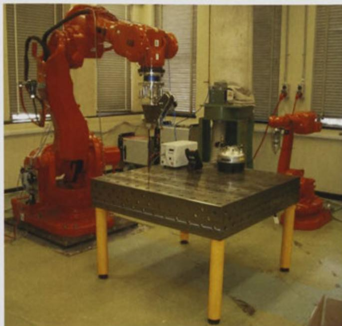
**Figure 39 – The ABB IRB6600 and ABB IRB1600 robot workcell.**
