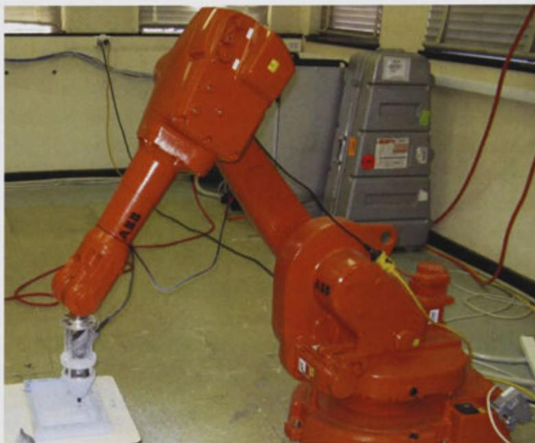
Figure 42 – Robotic milling setup of the ABB IRB1600 with spindle and foam sample
