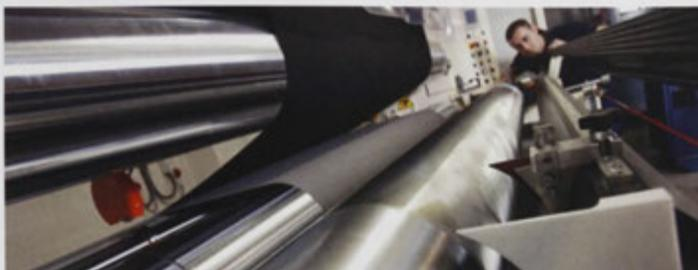
Figure 78 – Preimpregnating machine using hot melt and knife-coaters / filmers for resin coating
