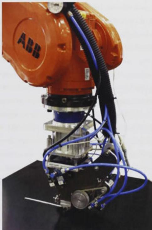
Figure 21 - UVAFP curing of a glass-fibre/vinylester composite.
