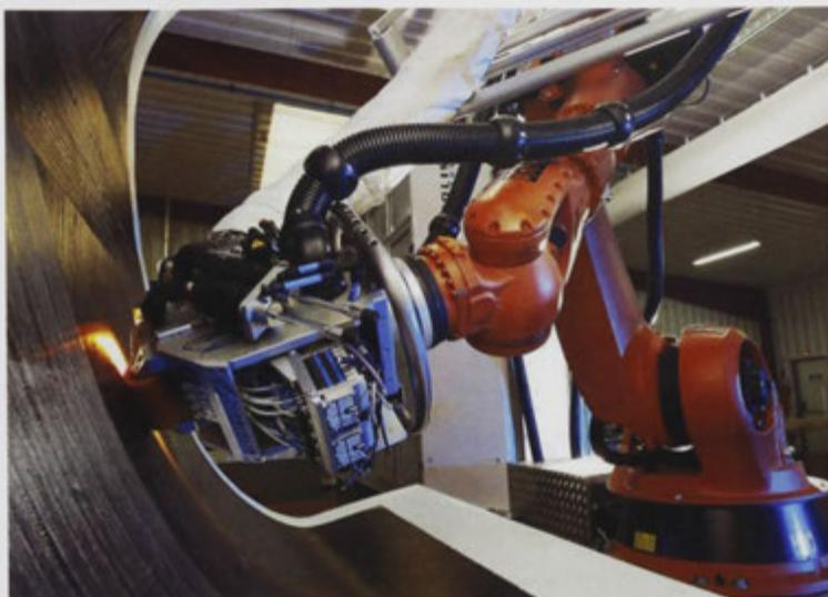
Figure 1 – An AFP system by Coriolis Composites
