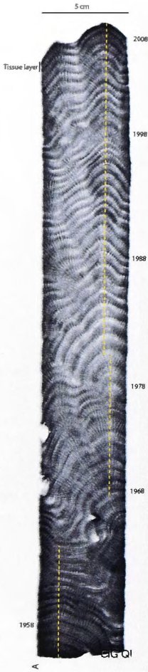
Fig. B-5 Positive print from X-radiography of coral slabs from Little Kindermar (LMI08-C-a) over the period 1956-2008. Chronology was reconstructed by cross checking of high density bands and Sr/Ca ratios from LA-ICPMS. Yellow dashed lines indicate the maximum growth axes which agree with tracks of LA-ICPMS.
