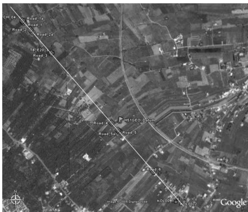
Fig. 8: The 2 km investigated course of the Roman road through the Helike plain. Excavation and resistivity tomography located the road at a length of 1.3 km between the locations Road 1 (west) and Road 6 (east).
