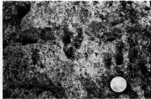
Figure 21 - Development of calcareous crust (white areas)
