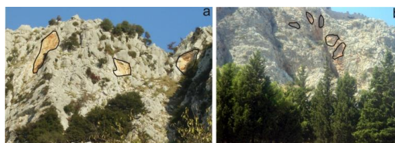
Figure 3 - Rock fall release areas in a) Skolis and b) Acrocorinthos steep rock slopes.
