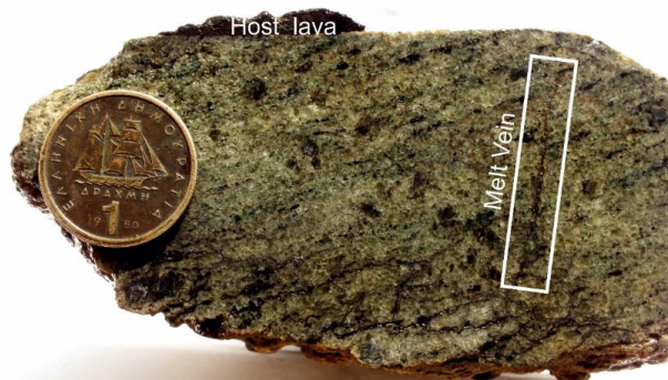
Figure 3 - Hand-specimen image of sample MA-1 xenolith from Taфраoute maar. A melt vein with phosphorus-rich olivines is indicated by the white rectangle.
