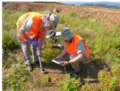
Figure 5 - Test measurements with the field spectrometer near Stratoni (Chalkidiki).
