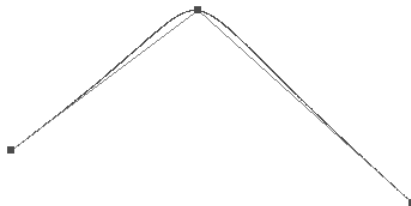
Figure 2: The quadratic trigonometric polynomial curve with \lambda = \sqrt{2} interpolates the control points, having end tangents parallel to the sides of the control polygon.
