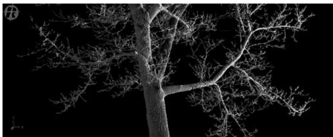
Figure 1: Merging point clouds. In that example darker points were obtained by scanning the tree from the left side and lighter ones were obtained from an opposite point of view. The two point clouds were merged automatically owing to reference targets located around the tree.
