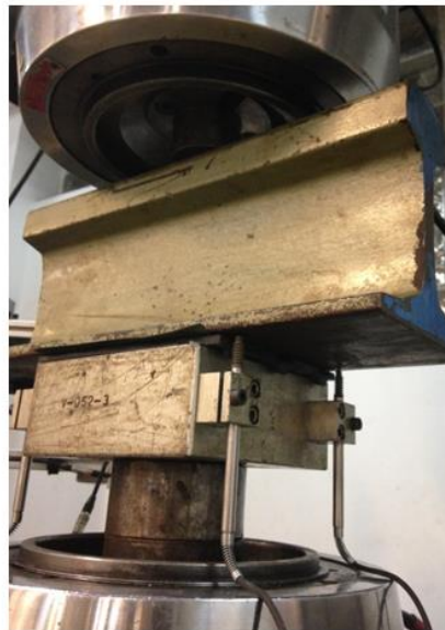
Figure 3.1. Assembly used for the stiffness tests
