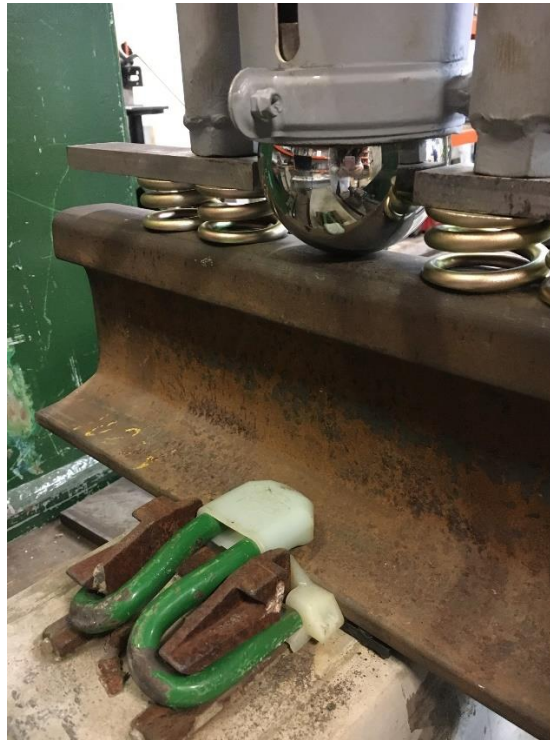
Figure 3.2. Impact testing arrangement
