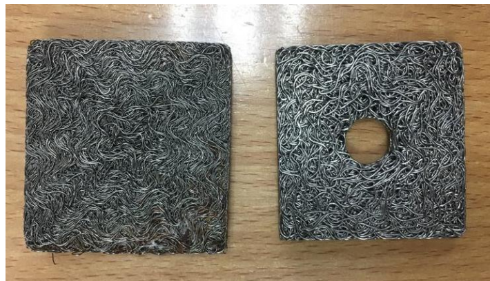
Figure 1.5. Pads made out of stainless steel.
