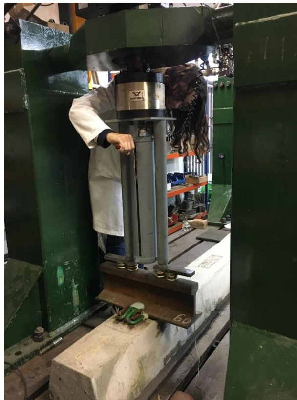
Figure 3.6. Testing using the alternative method with springs
