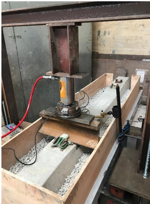
Figure 3.13 Verification of the deflection of the ballast
