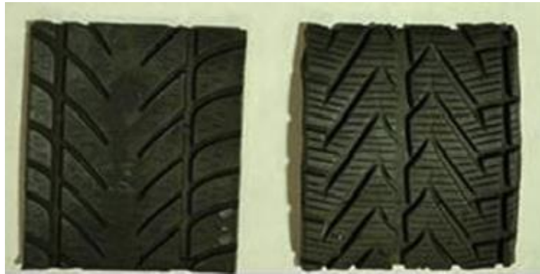
Figure 1.4. Pads made out of used tires [13].
