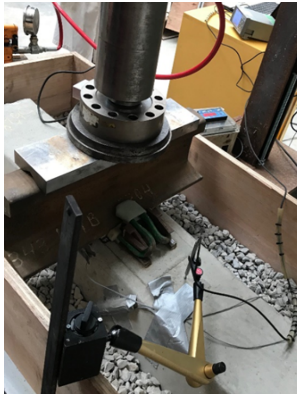
Figure 3.14. Detail of the LVDT Transducer
