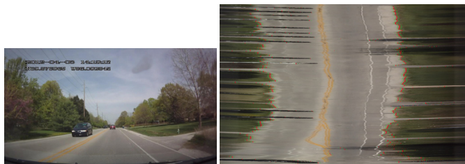
Fig. 7 The detected road edges in road profiles without using lane marks. Red bounded by two side green are detected road edges. High accuracy results in output outside road shoulder. Except some passing vehicles both the edge with close-to-horizontal traces, the road edges are located almost perfectly.
