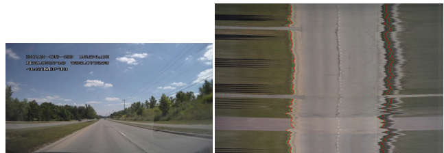
Fig. 8 Road edge detected at curb on right side. Left side without shadow causes the road edge detected at grass margin.
