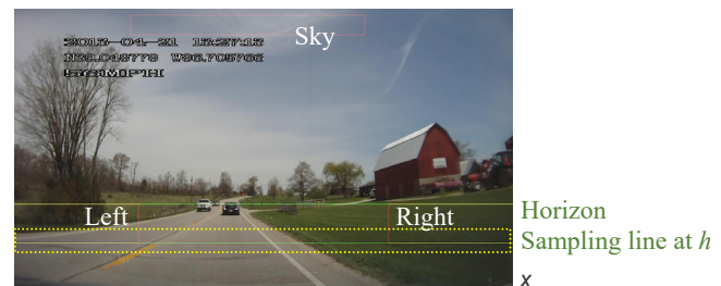
Fig. 1. Sample video frames for a road profile and weather data. Yellow belt around a sampling line is used to calculate the linearity of road edges. Weather sensitive data are sampled in three regions indicated in the image.
