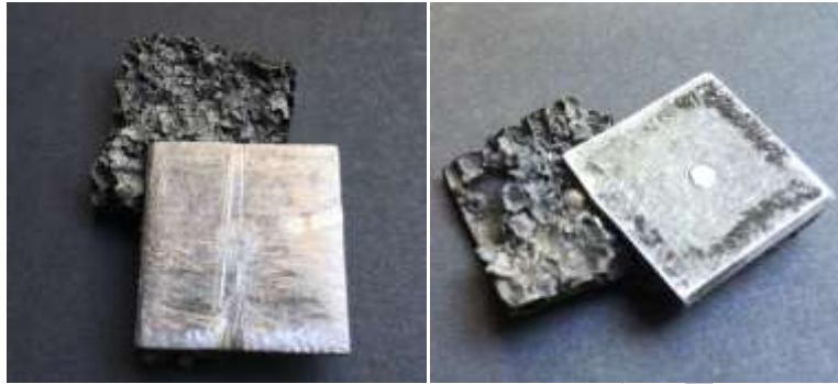
Fig. C. 1. Failure of the single-pinned AFS samples: the plates slide out of the compression axis.
