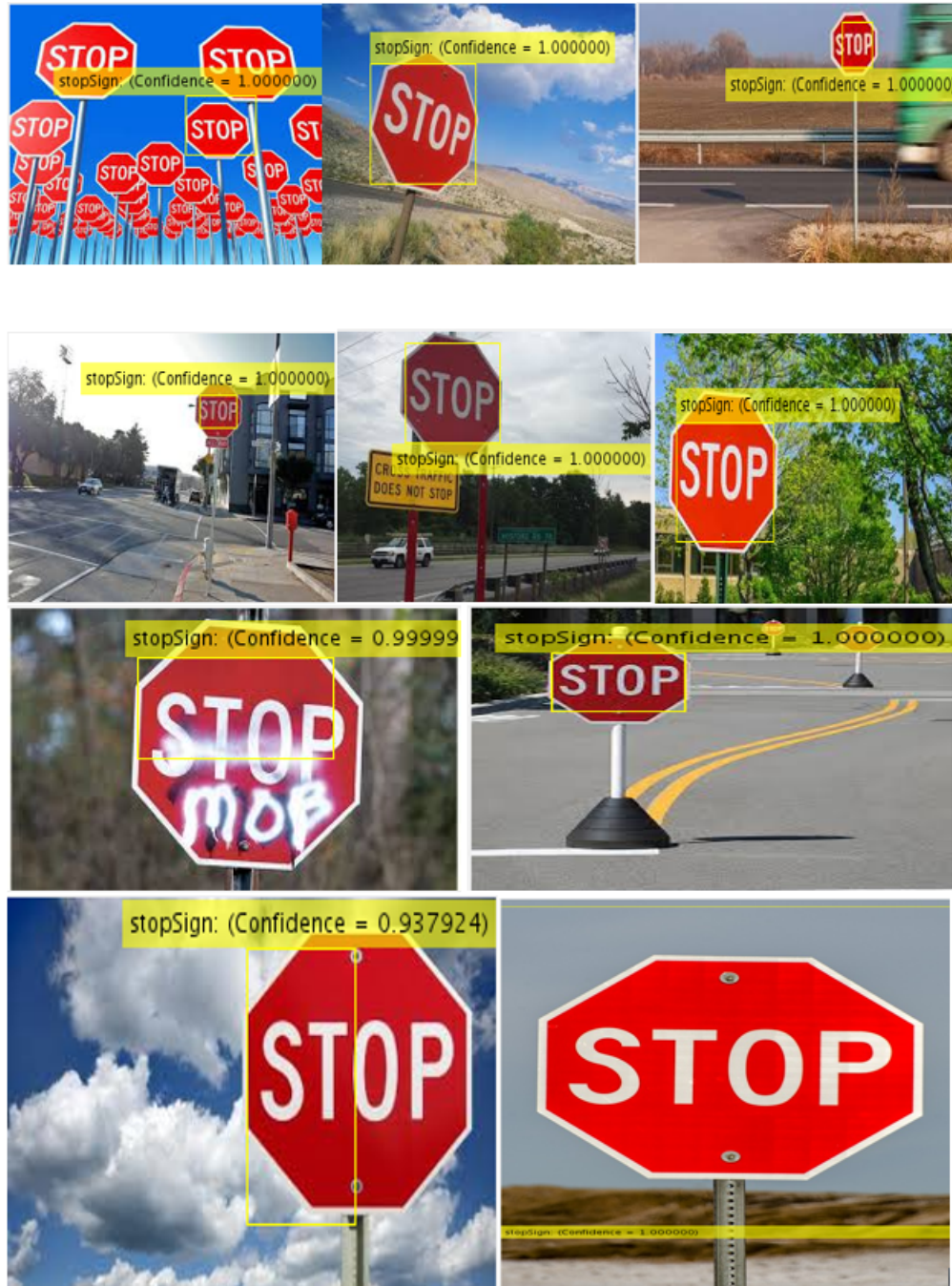
Fig. 2.12.: MATLAB detection with already trained network
