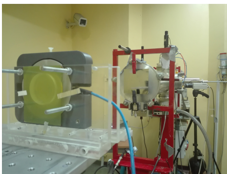
Figure 3. Picture of the experimental setup. An ionization chamber is placed between two PMMA supports on a moving table. A piece of Gafchromic EBT3 film is attached to the rear of the second PMMA support, after a circular collimator. The beam, coming from the front, traverses a tungsten scattering foil of variable thickness and approximately 50 cm of air, before reaching the ionization chamber.
