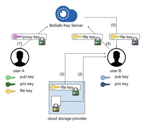
Fig. 7. BeSafe proxy re-encryption architecture
